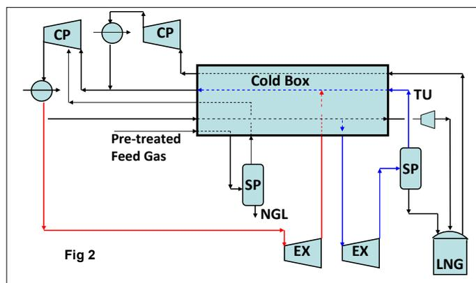
This configuration termed Integrated Pressure Liquefaction sees the feed natural gas, after liquids removal, introduced at an appropriate inter-stage point in the recycle gas compressor. This enables the liquefaction pressure to be set at a higher pressure than the feed gas without installation of additional compression plant with its associated capital and operating costs.
