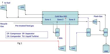
expanders by the recycle compressor CP1. Flash gas is also routed through the cold box and recaptured to the system by a small compressor CP2 which feeds the suction of the recycle compressor. The expanders are configured as companders and operate in series with the recycle gas compressor (Fig 2), recovering approximately 35% of the power required to run the system.
