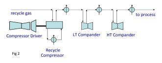
ZR-LNG is similar in concept to nitrogen schemes. However it enjoys a fundamental advantage as methane has a higher specific heat than nitrogen. This significantly reduces circulating flows which in turn reduces power consumption and pipe sizes.
