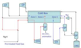
passing the feed gas plus recycle gas through the high temperature gas expander CX1 (Fig 4) and separating the condensed heavy material from the expander outlet at around 10-15 bar. This solution de-couples the vapour/liquid separation and feed gas pressures and saves a large part of the equipment and cost of a separate expander based NGL removal unit. It also reduces footprint which is particularly relevant to FLNG applications.
