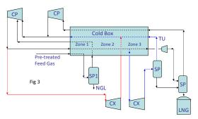
enhancing liquefaction efficiency without need for a separate feed gas compression plant.
