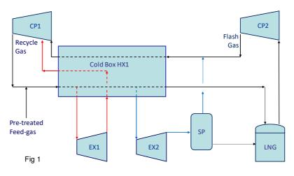
system by a small compressor CP2 and routed through the cold box to the suction of the recycle compressor for return to the expanders.
