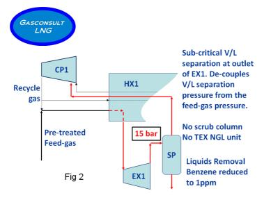
expander EX1 and separating the condensed liquids from the expander outlet at sub-critical pressure (see Fig 2). This IHR de-couples solution the vapour/liquid separation and feed-gas pressures and saves a large part of the equipment and cost of a separate expander based NGL removal unit. Specifically, the expander and re-compression facilities already exist in the basic ZR-
